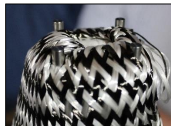
(Above: Example of loose tie off of braid to facilitate full fabric saturation)
