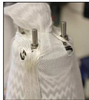
(Above: Example of split tape to veer around braid/features)
